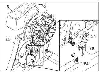
Then, remove all the screws from the Left and Right Front Shields (22, not shown); **there are three sizes of screws in the Front Shields—note which size of screw you remove from each hole.** Then, gently pull the Right Front Shield away from the frame.
